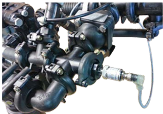
PRESSURE TRANSDUCER KIT PN# 53491
