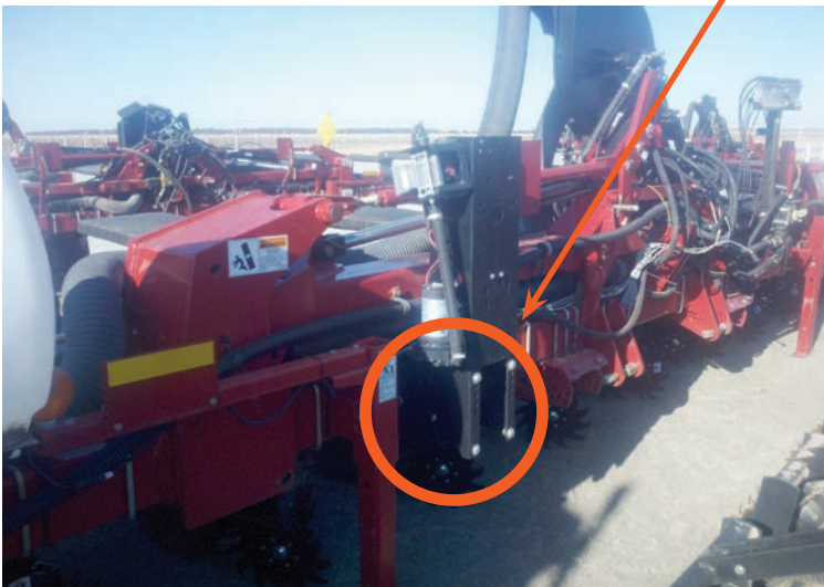
PN#55060 GX2 Extender bracket mount
