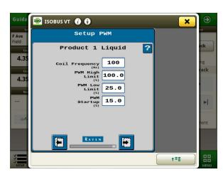
For best startup performance, set the PWM Startup at or slightly above the normal operating PWM Duty Cycle (DC%). When the pump starts it will go immediately to that Duty Cycle and then will have just a minor adjustment to lock on to the Target Rate. IF THE PUMP STARTS TOO FAST, LOWER THE PWM STARTUP.
