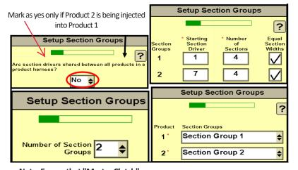
Note: Ensure that "Master Clutch" is not checked
