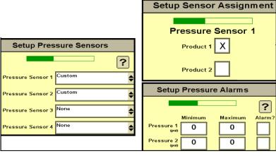
Sensors (such as pressure, pump RPM, spinner RPM) do not need to be assigned to a specific product if they are just being used to monitor a device and not to control it. AgXcel recommends that you NOT assign pressure and RPM sensors to a specific product. However, there may be times when you want to assign the sensor to a product.
