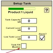
Check **Tank Fill Monitor** box if using a fill flowmeter. Then enter **Tank Fill Flowmeter Calibration (Units are 10 gal.)**
