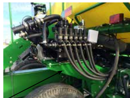
PN#54586 CASE IH/JD bracket to mount the GX5 on the draw bar (Bracket can fit draw bars 8" to 10" wide)
