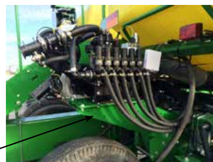
PN#54397 GX5 Bracket for JD1720 CCS (mounted to circular plate on lift assist frame)
